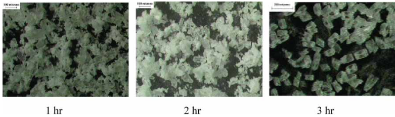
Figure 7. Photos of the crystals obtained by evaporative crystallization with elapsed time.
